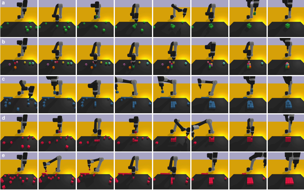
Figure S4: Snapshots of the task “build \{i * j * k\} {structure}”. (a) Build a 2 \times 2 \times 2 cube. (b) Build a 3 \times 2 \times 2 pyramid. (c) Build a 4 \times 3 \times 3 pyramid. (d) Build a 1 \times 3 \times 3 wall. (e) Build a 4 \times 4 \times 1 base.
