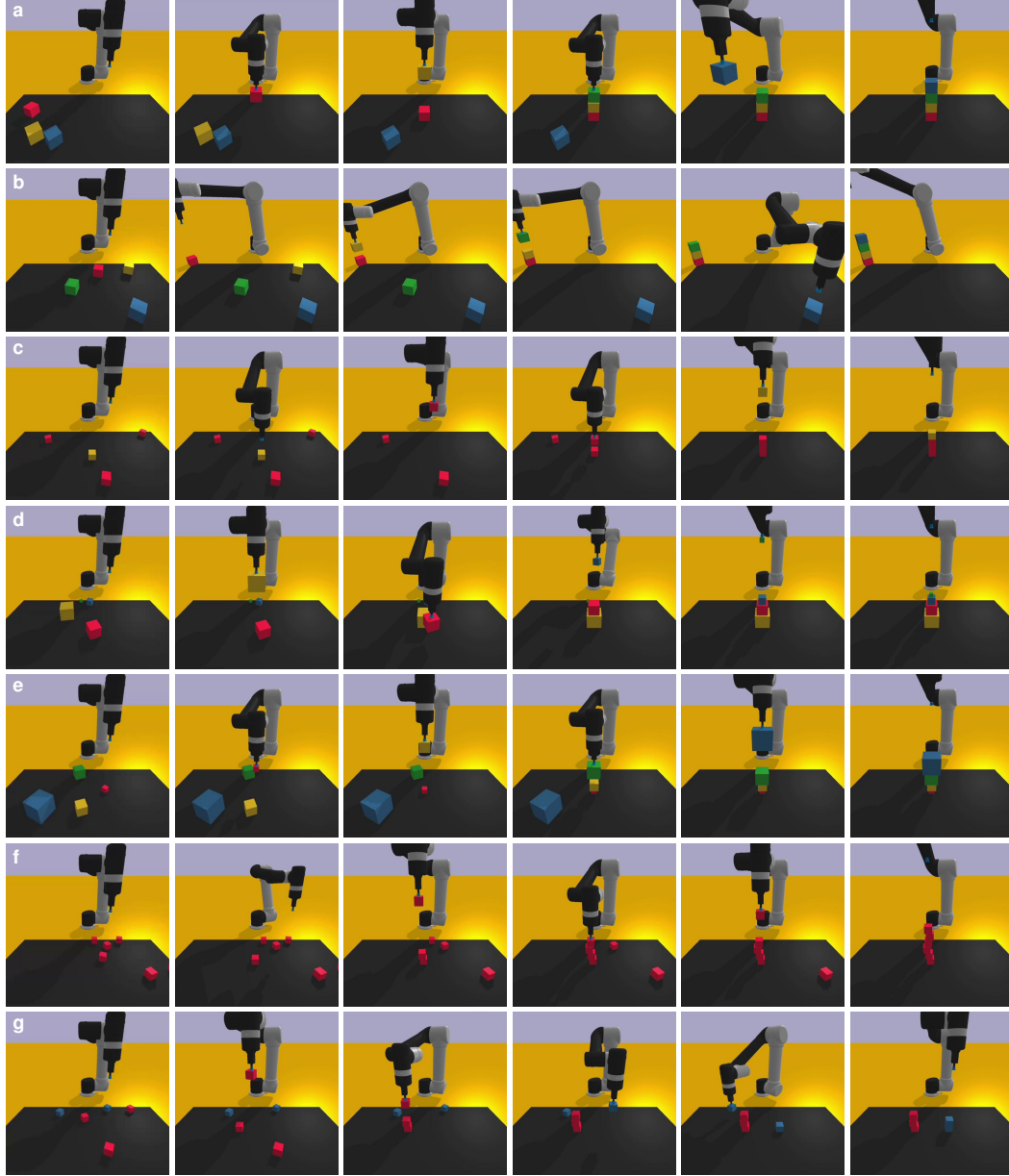
Figure S2: Snapshots of the “stack blocks” task and its variations under user-guided lifelong learning. (a) Stack 4 blocks corner-to-corner at the workspace center. (b) Stack 4 blocks with a 45^\circ rotation at the back-right table corner. (c) Stack blocks by color, with the yellow block on top. (d) Stack blocks from largest to smallest. (e) Stack blocks from smallest to largest. (f) Stack blocks into a zigzag tower. (g) Build two towers sorted by color.
